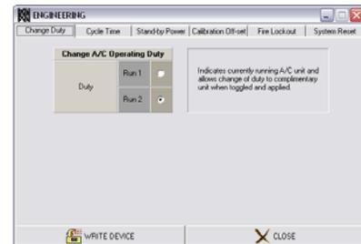
15. In the Engineering/Change Duty window, the currently active air-conditioning unit in operation is displayed and if required, it can be toggled to change to the complimentary unit.
